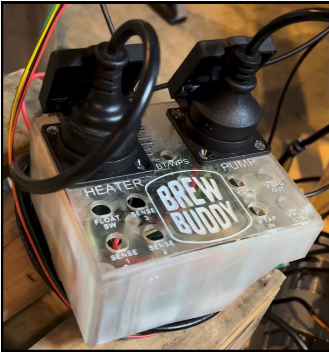
Figure 5.7 Brew Buddy Enclosure Printed
