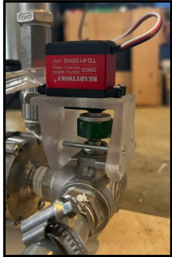
Figure 4.21 Servo Valve
